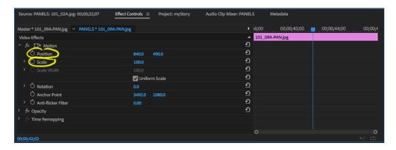
For purposes of moving the camera we are concerned with the "Position" and "Scale" coordinates. Position to pan your camera up, down, or a combination of the two. Scale in order to zoom in and out. You can control these coordinates by either moving the panel in the Program window (as we did in the previous step) or by clicking on and changing the numbers directly in the Effects Control window.
